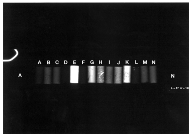
Figure 1 Radiograph of various cement preparations from which optical density measurements were made. Specimens are organized alphabetically, although only the first and last specimens in each row are labeled. A = Simplex P; B = Simplex P plus 20% by weight BaSO 4 ; C = Mathis; D = Cranioplastic plus 10% by weight BaSO 4 ; E = Fixos; F = Chemfix3; G = Orthocomp; H = Murphy; I = Olan; J = Simplex P plus 30% by weight BaSO 4 ; K = Deramond; L = Cranioplastic plus 20% by weight BaSO 4 ; M = Jensen; N = Cranioplastic plus 30% by weight BaSO 4 .
